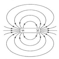
Take the central axis through the north and south pole (indicated by N and S) to be the z axis and call the two-dimensional cross section of the bar magnet orthogonal to this central axis the base.
